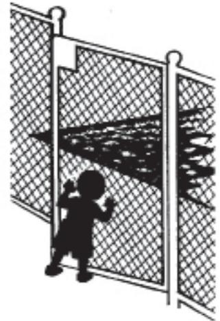
7. Where the barriers composed of diagonal members, such as a lattice fence, the maximum opening formed by the diagonal members shall not be more than 1.75 inches (44 mm).
