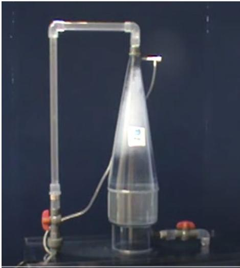
**Figure 1.** Speece Cone with bubble swarm in top of cone dissolving into water by the bottom of the cone. The oxygen feed is at the top of the cone. Note the bubble swarm trapped in mid-cone. Screenshot from <https://www.youtube.com/watch?v=6thCFEWSrw>.
