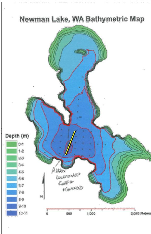
Figure 9. Example layout of a 2,000 ft line diffuser in Newman Lake
