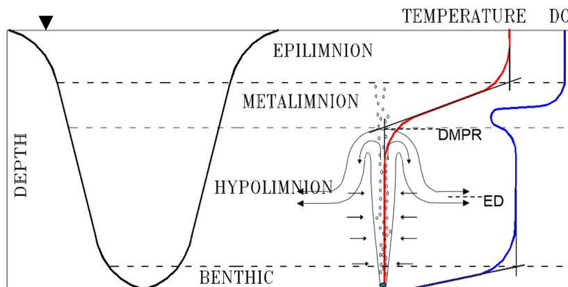
Figure 7. Schematic showing water column regions based on thermal structure with plume overlay showing example of circulation. Blue line represents a typical oxygen profile and red line represents a typical temperature profile. DMPR is the depth of maximum plume rise and ED corresponds the equal density layer plume water falls back to.
