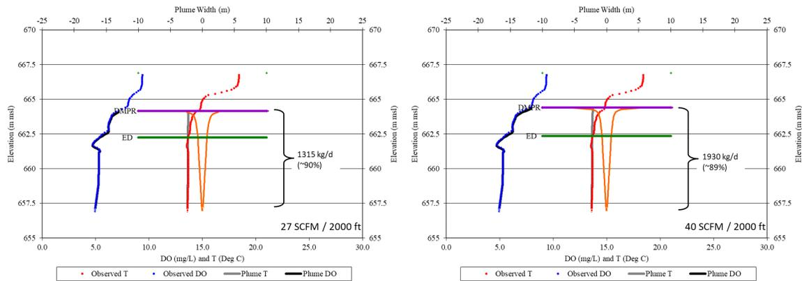
Figure 10. Example of plume model predictions for 27 and 40 SCFM applied gas flow rates for May 28, 2014 data set. Blue and red data points represent observed dissolved oxygen and temperature data respectively. Black and gray lines represent model predictions for dissolved oxygen and temperature respectively. Orange lines represent plume width and the purple and green lines correspond to DMPR and ED respectively.
