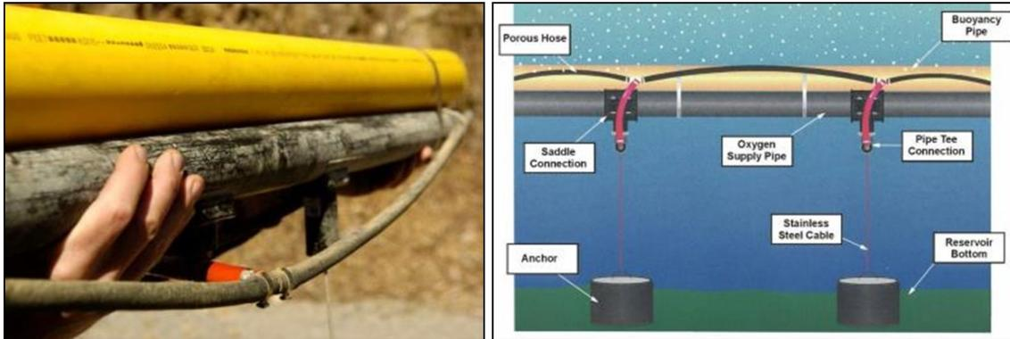
Figure 8. Line diffuser section (left) and deployment schematic (right).
