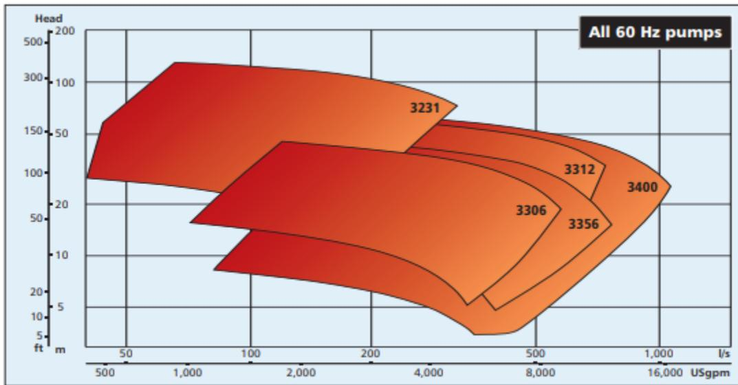
Figure 2. Flygt 3306 pump composite curve.
