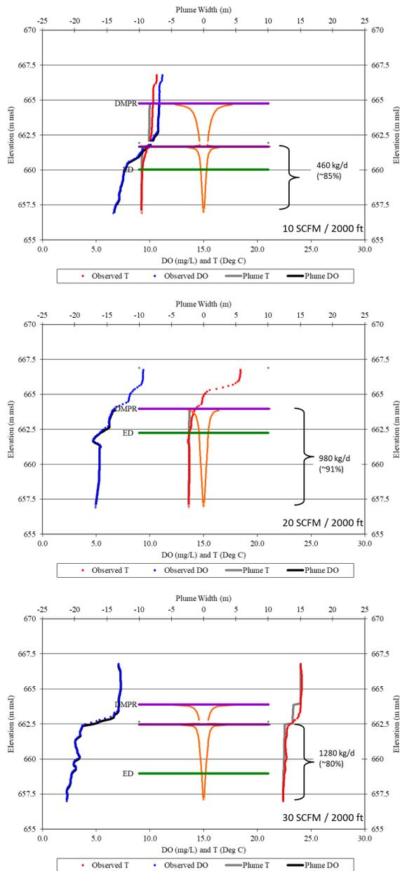
Figure 11. Example of plume model prediction for 10, 20, and 30 SCFM applied gas flow rates on April 22 (top), May 28 (middle), and August 12, 2014 (bottom) respectively.
