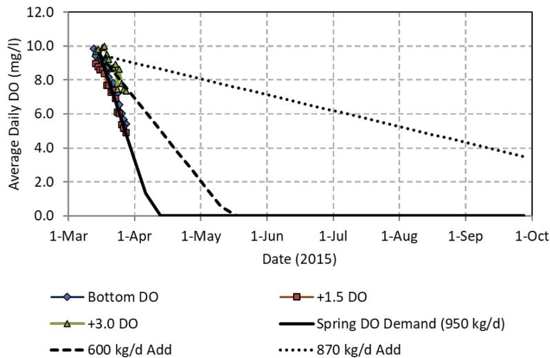
Figure 5. Remote data collected in March 2015 showing dissolved oxygen (DO) data, average depletion rate per the data (solid line) of 2,100 lb O<sub>2</sub>/day (950 kg O<sub>2</sub>/day) and predictions for 1,320 (dashed line) and 1,923 (dotted line) lb O<sub>2</sub>/day (600 and 870 kg O<sub>2</sub>/day) oxygen addition rates. Data points are from Figure B4 (Appendix A) and represent data collected 0.1 (red squares) 1.5, (blue diamonds), and 3.0 (green triangles) meters above the bottom.
