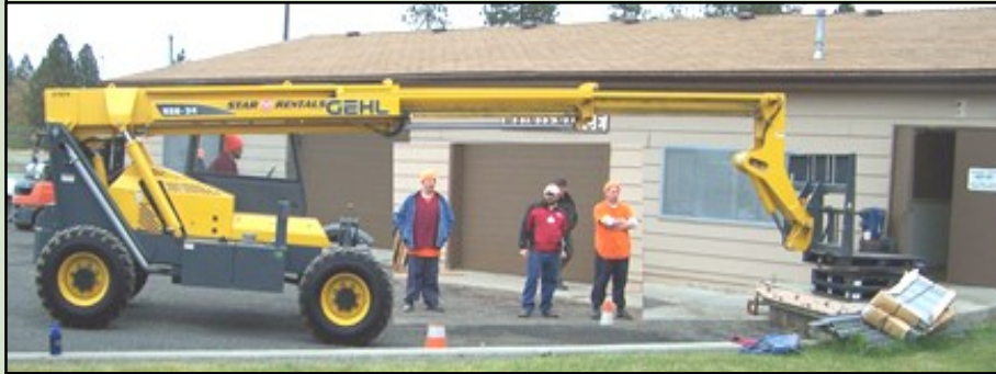
Geiger inmates participating in AGC Pre-Apprenticeship training shown practicing with Class VII rough terrain forklift.
